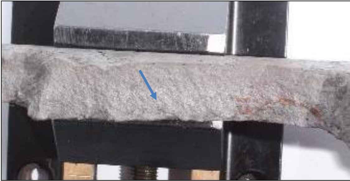
Figure 3 (b): Expanded area gathered from Figure 3 (a) displaying the direction of crack propagation.
