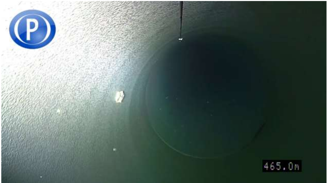
Joint image with possible gasket identified
