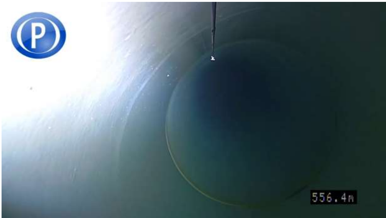
Joint image with possible gasket identified
